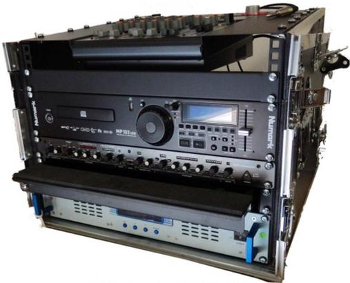
This photo shows the latest version of Proteus (Radio-in-a-Box) that is built for a customer in the Pacific. Since the application is as a portable radio station, the system includes a Pelican case to carry sensitive peripherals such as microphones, monitor speakers etc.
